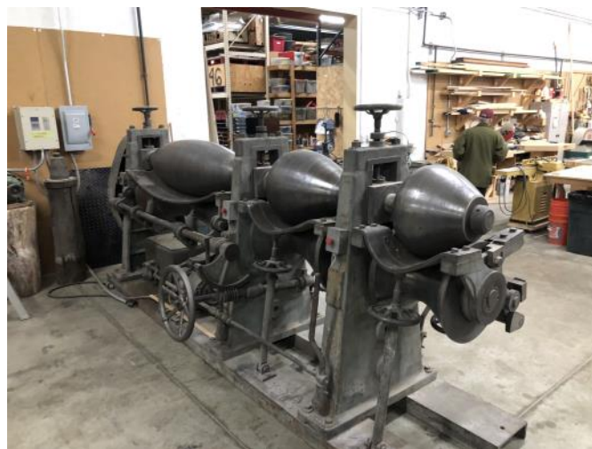
David Cooper explained how the French used this Swiss-made metal former (above) to create shapes like the fender of the Talbot Lago coupe (left) in only a few passes. It was the French body builders' "secret weapon," allowing them to create complex shapes more quickly.
