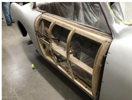
The shop has a complete woodworking section, needed for this Bugatti sliding roof (above and left), and this Talbot Lago door frame (below). Woodworker Bob Ludwigson was impressed.
