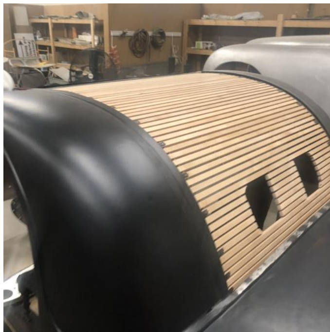
The shop has a complete woodworking section, needed for this Bugatti sliding roof (above and left), and this Talbot Lago door frame (below). Woodworker Bob Ludwigson was impressed.
