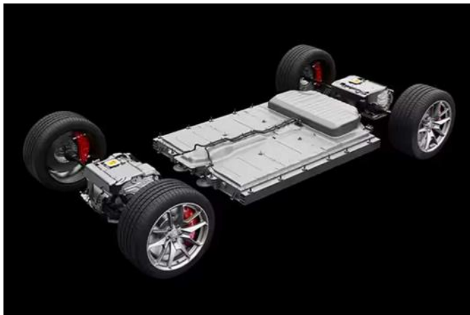
Dodge Charger electric motors and battery
