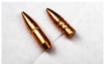
Boat-(l) and flat-tail bullets
