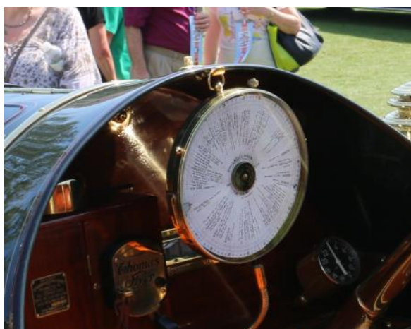
Perhaps the world's first nav system, the dial on this 1910 Thomas Flyer contained route instructions. The pointer was connected to the transmission by a flex shaft to track mileage.
